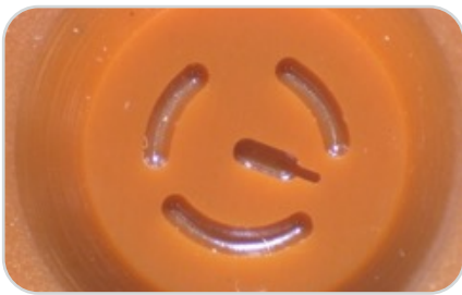
Figure 7, The Spark rotor seal shows some superficial wear after 30,000 injections. The stator shows no wear after 90,000 injections. There are no consequences for the analytical performance
