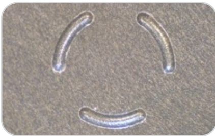
Figure 8, The Vendor A rotor seal and stator show some traces, but they have no consequences for the analytical performance
