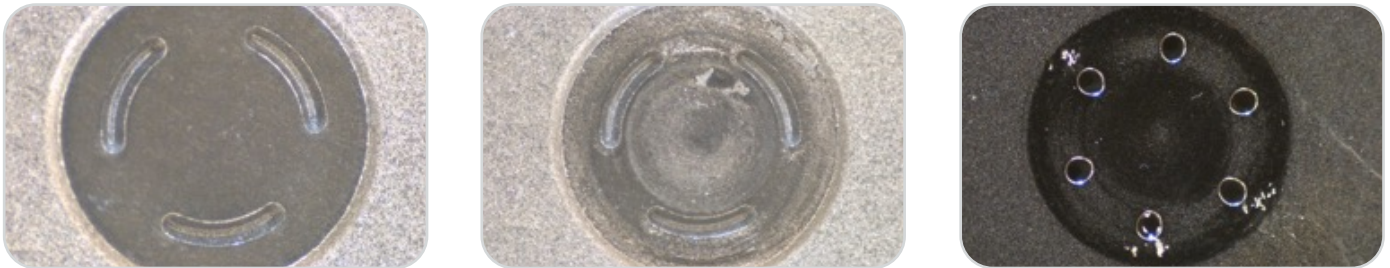
Figure 9, The Vendor B rotor seal shows some light wear on the low pressure side and the stator shows a damaged coating, but they have no consequences for the analytical performance
