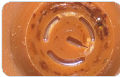
Figure 7, The Spark rotor seal shows some superficial wear after 30,000 injections. The stator shows no wear after 90,000 injections. There are no consequences for the analytical performance
