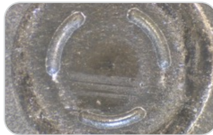
Figure 8, The Vendor A rotor seal and stator show some traces, but they have no consequences for the analytical performance
